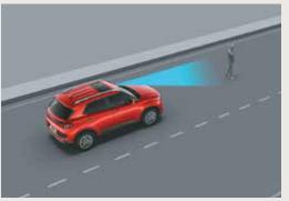
Forward Collision - Avoidance Assist - Pedestrian (FCA-Ped) Forward Collision - Avoidance Assist - Cycle (FCA-Cyl)
