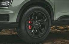
Black painted alloy wheel with red front brake caliper
