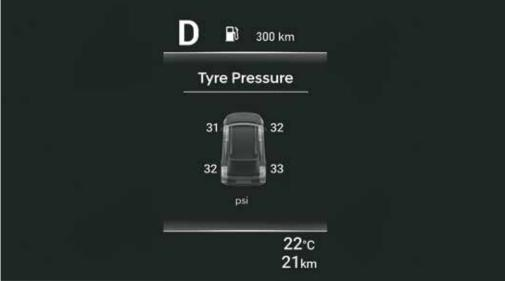
Tyre pressure monitoring system (Highline)
