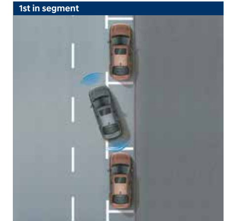
Parking assist (front & rear parking sensors and rear camera with dynamic guidelines)
