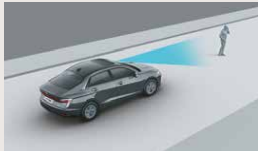
Forward Collision - Avoidance Assist - Pedestrian (FCA-Ped)
