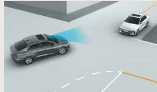
Forward Collision - Avoidance Assist - Junction Turning (FCA-JT)
